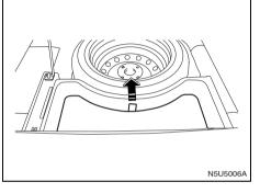
6) To access the tools, pull the strap on the tool box cover upward. The tools are located inside the foam tray.
